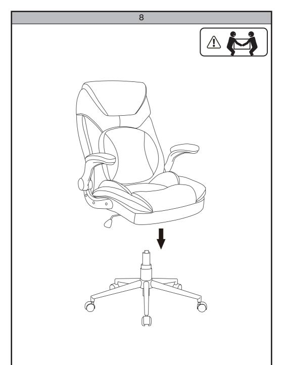
Align the hole underneath the chair with the gas lift cylinder. Press the seat down to secure the chair to the gas lift cylinder.
